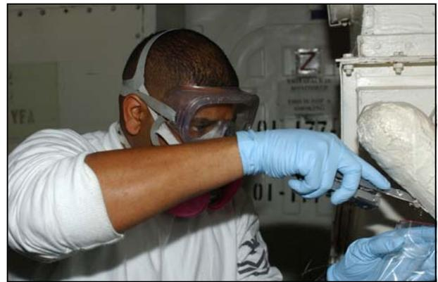
A damage controlman collects samples of lagging from a shipboard space to see if there are traces of asbestos aboard.
