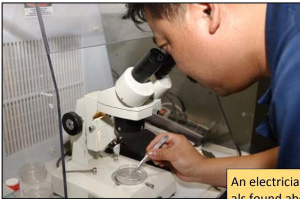
An electrician’s mate conducts asbestos checks on materials found aboard a carrier. Such regular monitoring maintains safety and health standards for every Sailor aboard.
